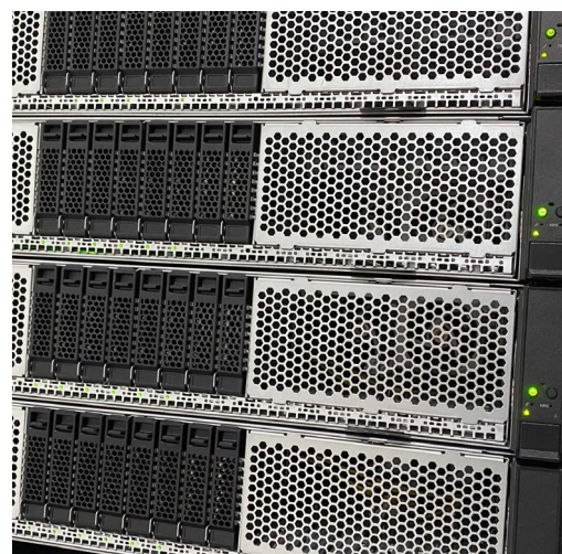
© 2022 Olympic Broadcasting Services Together with Intel, OBS has set up a virtualised OB van at the National Aquatics Centre to explore new ways of producing the coverage of the Olympic Games. In this new environment, all the standard broadcast hardware such as the video mixer have been replaced by software running in the cloud.
